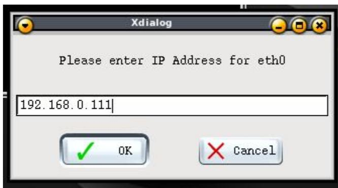
Figure 14 – Enter the host's static IP address
