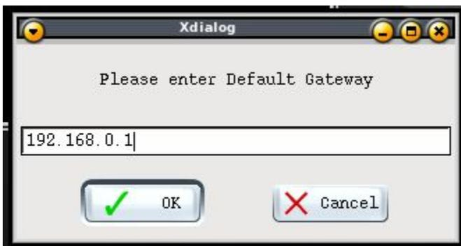
Figure 17 – Enter the host network's default gateway address – should be the same as the target's
