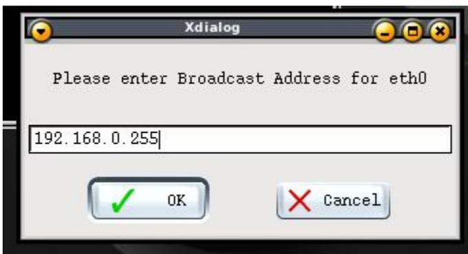
Figure 16 – Enter the host network's directed broadcast address
